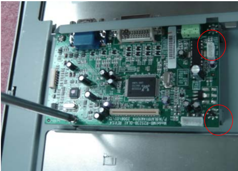
16. ( Take down the screws of main board & then take down the main board)
