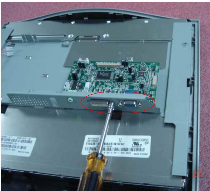
16. ( Take down the screws of main board & then take down the main board)
